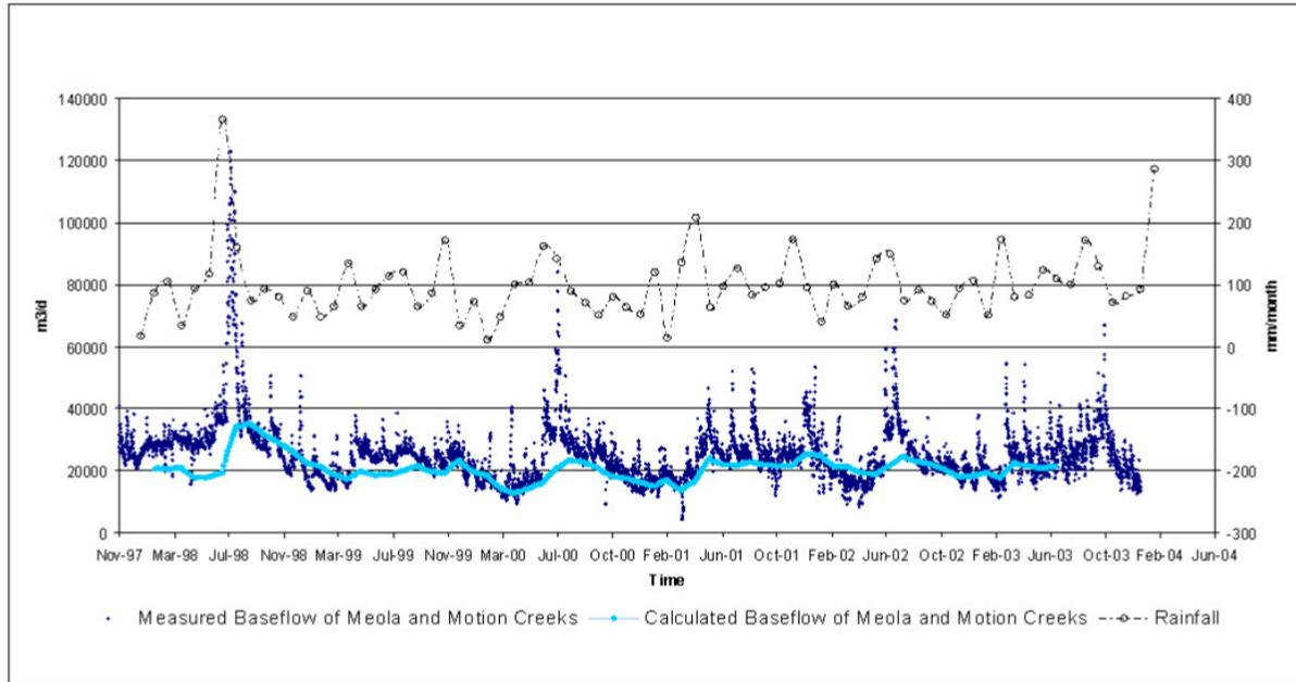
**Figure 4. Comparison of Monitored and Modelled Groundwater Discharge (Baseflow) (PDP 2005b)**
